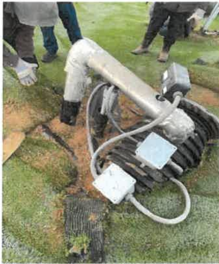
Figure 9. Settlement induced wrinkles and torn ClosureTurf® at leachate piping on south slope
